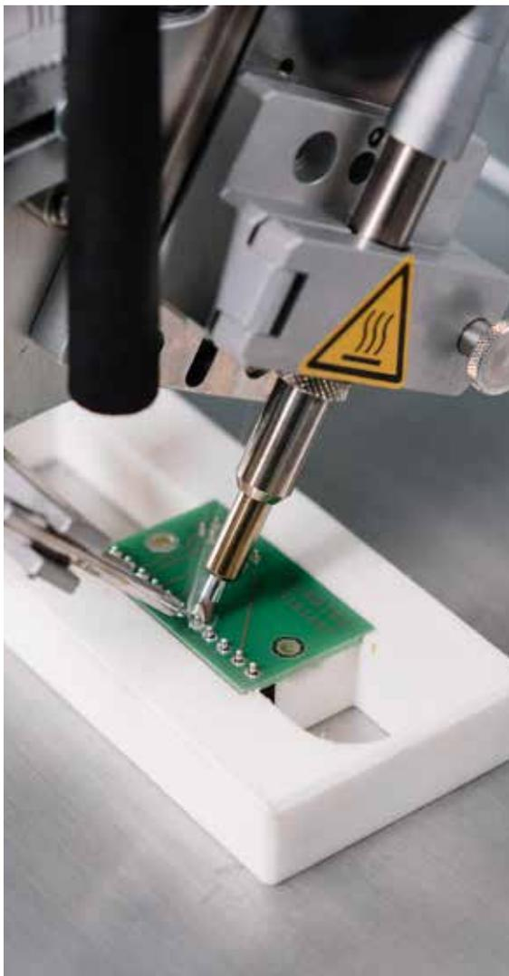
Optimal soldering requires a process in which all parameters involved can be individually configured. These parameters must be consistent and precise for all soldering jobs. This is the only way to ensure that there are no fluctuations in the quality of the solder joints.
