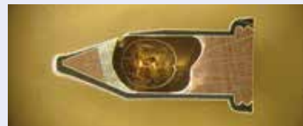
Micro-section of soldering tip with hole formation
