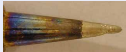
Soldering tip after 10,000 solder joints with lead-free SA
