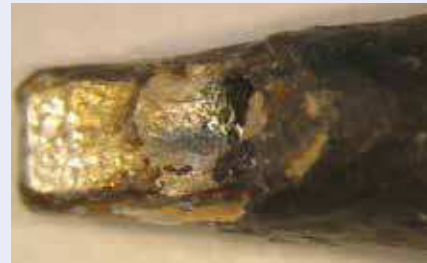
Formation of holes in the soldering tip
