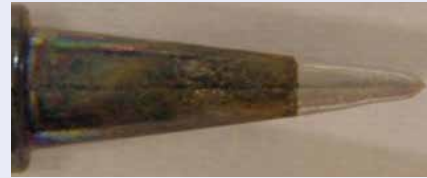
Soldering tip after 20,000 solder joints with Sn60
