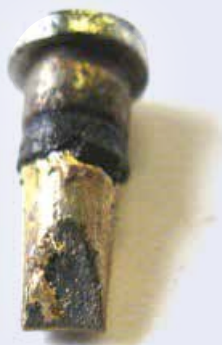
Oxidation of the Soldering Tip
